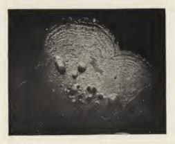
Fig. 26. (x 15 Diameters. Oblique Illumination.) Section of Knob of Electrolytic Nickel.
